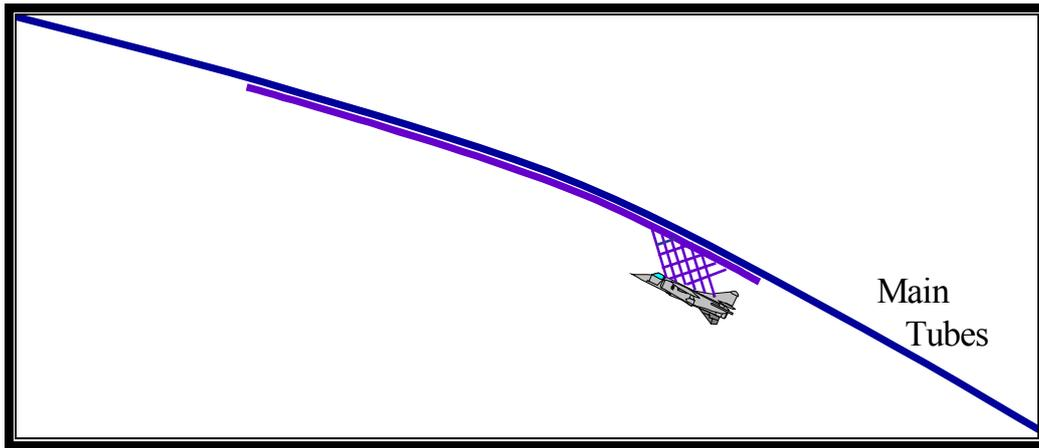
**Figure 6 Bearer supporting a vehicle during launch**
