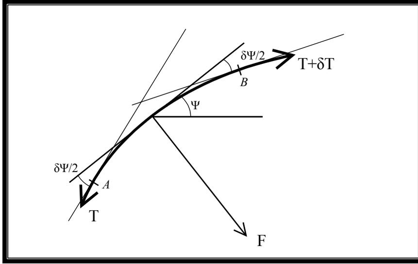
**Figure 2 Forces over a small segment  $AB$  of the tube**
