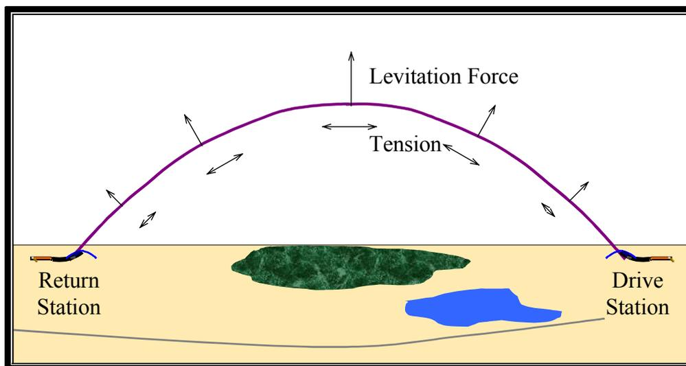
Figure 1 Shape of Curve indicating Tension and Normal Forces
