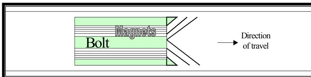
**Figure 3 Scoop at front of bolt**
